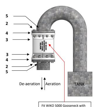
Check classification rules if a screen is needed when the air pipe head is fitted on a ballast tank. If not, remove the screen when the air pipe head is fitted on ballast tanks
